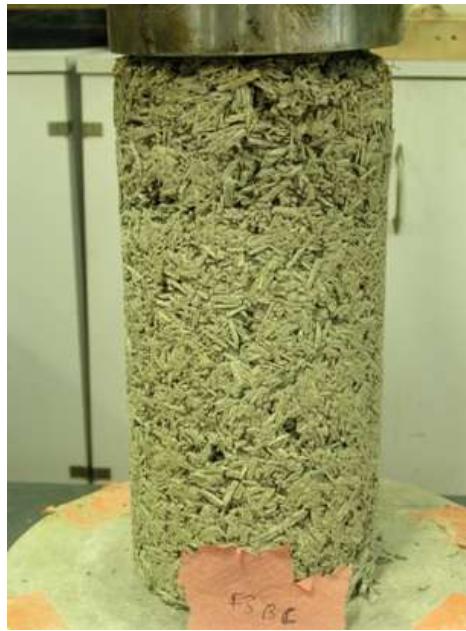
Fig. 4. Hemp sample during the compressive strength test.
