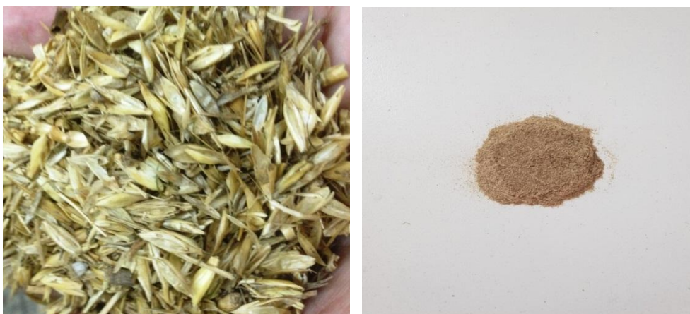
Figure 1. Wheat husk (WH) before and after grinding.
